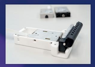
The holder is used to precisely position and analyze PCR tubes in front of the detector.
