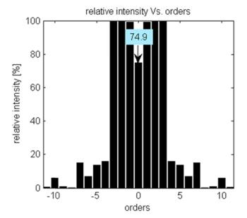
In the above examples, the zero order after some manufacture errors is 1.57% of input beam in case of MultiSpot 1x6 (left picture) and 74.9% of other desired orders average in case of MultiSpot 1x7 (right picture).
