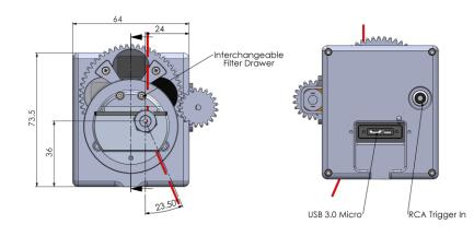
Optical distance from Input plane  $\boxed{A}$  to Detector Plane: 49 ±0.5
