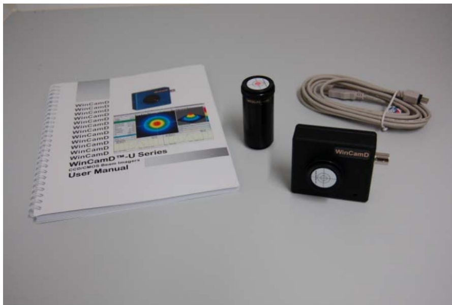
WinCamD, WCD-LPF1290 long pass filter, CM-50 50 mm tube,
