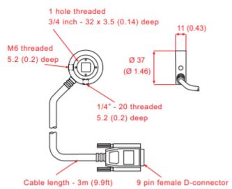
Dimensions are in millimeters
