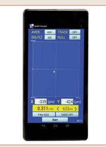
\* To maintain full calibration accuracy, attenuating optical filters may be necessary for operation with beams greater than 1 mW. Saturating "non-linear" effects depend on the beam size, type and wavelength, but caution should be exercised when using the PSD above 1-3mW.
