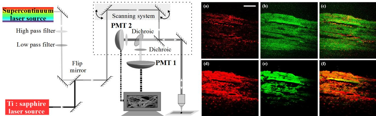
Figure 1. Left: Experimental setup. Right: sample images; a-c. Supercontinuum excitation. d-f. Ti: Sa excitation. Red color: TPF of Alexa Fluor; green color: SHG of myosin. Scale bar: 100  $\mu\text{m}$ . 40  $\mu\text{s}/\text{pix}$ ; 512x512 pixels.
