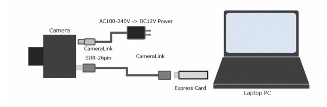
For the connector of this camera is SDR-26pin, please use the supported cable.
