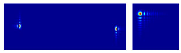
An Airy beam is a non-diffracting waveform which doesn't spread out as the beam propagates and gives the appearance of curving as it travels.
