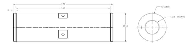
Internal SM1 threads on both sides of the module
