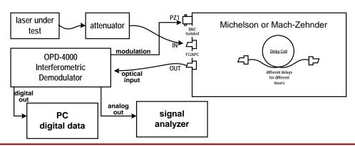
Laser under test is input to interferometer, which is set to the appropriate optical path mismatch by selection of the delay line which may be user installed or changed. OPD-4000 modulation output is applied to the PZ1 fiber stretcher input. **OPD-4000** phase measurement output is selected as either digital or Digital data is post analog. processed. Analog data is available to signal made analyzer.
