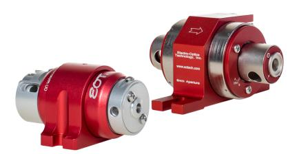
EOT's EURYS Broadband Rotators rotate the plane of polarized light 90° at 800 nm in the forward direction and 0° from 720 nm to 950 nm in the reverse direction while maintaining the light's linear polarization. When placed between crossed polarizers, a broadband Faraday rotator becomes a broadband optical isolator.
