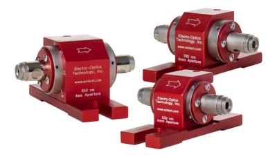
EOT's TORNOS Faraday Rotators rotate the plane of polarized light 45° in the forward direction and an additional 45° of nonreciprocal rotation in the reverse direction while maintaining the light's linear polarization. When placed between crossed polarizers, a Faraday rotator becomes an optical isolator.
