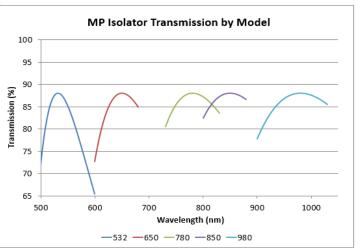
$<sup>^{\</sup>rm a}$  When placed between crossed polarizers having an extinction ratio of  $\geq$  1000:1
