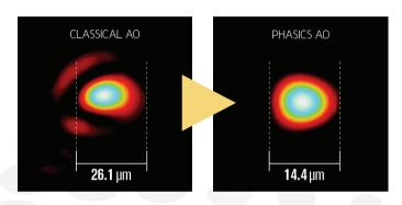
↑ Correction after the last parabola without any additional device to achieve the best possible focal spot
