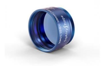
The beam shaper SQM25-10-D-A-532 generates from Gaussian laser beams in combination with a focusing lens a multitude of squared Top-Hat profiles in the focus area. Due to its high-precision mount, the a|SqAiryShape is always perfectly aligned and can be easily integrated into existing application setups thanks to its short overall length and convenient asphericon thread.
