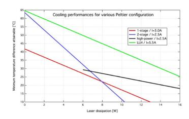
The HHL can be equipped with either a single-stage, double-stage or high power TEC cooler. Their performance are shown here and compared to the much larger LLH for reference. The single-stage and double-stage are equivalent in price and the ideal one will be chosen to fit the laser expected usage; the high power TEC is more expensive.
