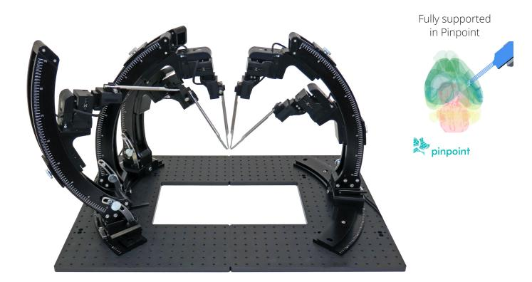
Clearly readable angle scales make angle adjustment in elevation and azimuth easy and reproducible - for up to dozens of probes.
