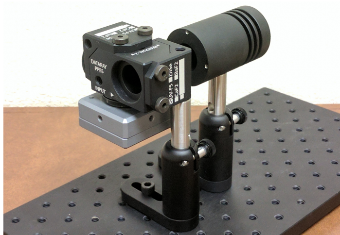
Figure 2: Polarization Preserving Beam Sampler with a WinCamD-LCM attached to Output and a Beam Trap behind Residual 1
