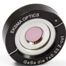
GaSe crystal mounted in Ø25.4 mm holder
