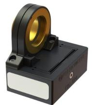
Nanopositioner dedicated to accurate positioning of microscope objective (stability in the picometer level). Used with Z-stack, automated focus or automated thermal expansion compensation.
