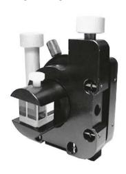
Continuously Variable Attenuator/ Beamsplitter is designed to be used for laser pulses as short as 100 fs. It consists of 2 highperformance polarizing optics components placed in precision opto-mechanical holder 840-0197. Variable attenuator/beamsplitter incorporates a high-performance Polarizing Cube Beamsplitter which reflects s-polarized light at 90° while transmitting p-polarized
