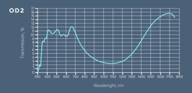
For optional use at higher than about 200 mW lasers (@1064nm) (does vary with wavelenght, refer to spectral sensitivity curve), you may consider using following filters to avoid sensor overfilling ("light flooding") issues and still ensure high visibility of your surroundings as the filter maintains high transmittance in the visible region compared to regular neutral density filters.
