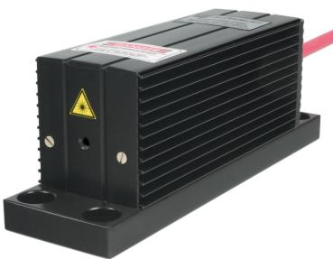
wide range of passively Q-switched lasers with pulse durations below 1 ns and extremely high peak powers at 1064 nm with excellent TEM<sub>00</sub> beam profile are offered by ALPHALAS. The PULSELAS®-P lasers feature proprietary microchip design. The monolithic laser cavity is permanently aligned and therefore extremely stable.
