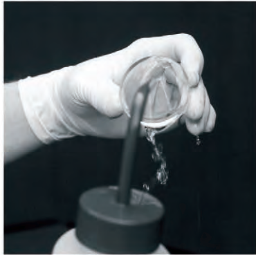
Figure 1. Flushing the optic with Vertrel XF or Asahiklin AK-225.
